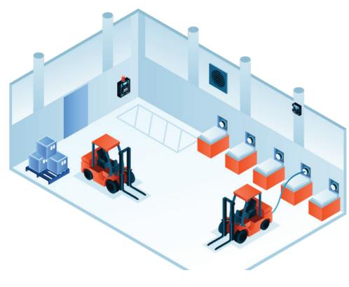
mounted on or near the ceiling above the battery charging area, where hydrogen gas will concentrate. Care should be taken to make sure the sensor is away from ventilation fans and any rapidly moving air.
