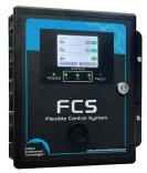
The FCS-32 is a sophisticated, high performance system controller that offers up to 32 gas channel configurations for monitoring toxic, combustible or refrigerant gases with versatile control functionality for non-hazardous, non-explosion rated, commercial and light industrial applications. The FCS -32 is designed to accept inputs from digital and/or analog transmitters and/or Peripheral Devices (in various combinations), using Modbus® RTU RS-485 or 4-20 mA analog input.
