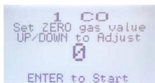
Attach the regulator to the cylinder of zero air, insert calibration adapter into the sensor opening on the front of the enclosure door (see Section 7.3.1 *Calibration Adapter Plug* if the adapter will not fit). Press Enter to start the Zero calibration. The display will show a countdown from 18 seconds.
