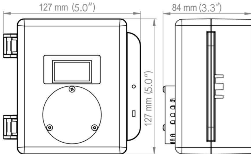
Above dimensions are shown with optional splash guard. Without splash guard, thickness is 71 mm / 2.8 in. The area required for enclosure door to be open 90 degrees is 178 mm / 7.0 in or 254 mm / 10.0 in for fully open. With the optional splash guard installed, the enclosure is IP54 rated.
