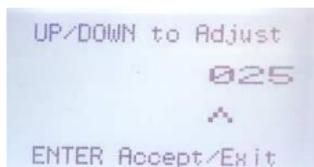
**NOTE:** An Ascending alarm is used when the normal gas level starts out below the alarm setting and when the reading goes above it, the alarm will trip. A descending alarm is used when the normal gas level starts above the alarm setting and when the reading goes below it, the alarm will trip. The descending alarm is commonly used with Oxygen sensors.
