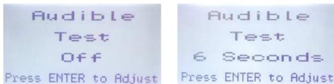
Move to the next digit by pressing ENTER. When finished, press ENTER to save and Exit. The test will start immediately and will continue for as long as the time was set. The remaining time of the test can be seen counting down on the display. You can exit the menu without affecting the time. **If you want to end the test before the time is up, you must re-enter the Test Mode and enter a value of "0000" for the test length of that function.**
