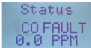
**NOTE:** While faults in the circuitry can be detected, a dead or damaged electrochemical sensor will usually appear to the transmitter as a zero gas reading. To ensure safe operation, periodic bump tests are required.
