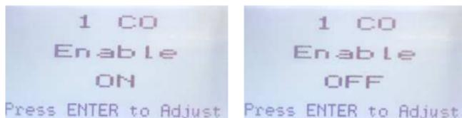
Press ENTER and use the ARROW key to scroll to the Enable screen. Use the ENTER key to choose ON or OFF. Use the ARROW key to move on to the next menu item and ENTER to Exit.
