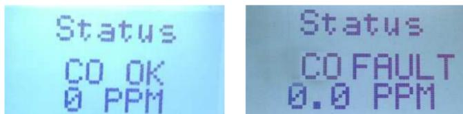
If the LPT-B is part of a system, such connected to a QCC or FCS, each gas channel splash screen will show the current status of the channel:
