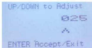
When finished, press ENTER to accept and Exit the screen. The gas level reading for that channel will be immediately sent to the controller. This test reading will override any actual gas reading for that channel for the duration of the test.
