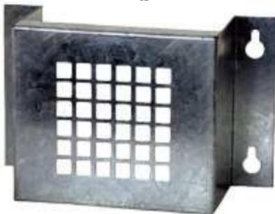
The metal protective guard is made of heavy duty metal and helps to protect against abrasive damage, theft and vandalism to the transmitters. It is made from 16-gauge galvanized steel and has 13 mm (½") square openings in the front to allow gas and air to flow through to the sensor. With only four slotted mounting holes, installation and removal for equipment servicing is easy.
