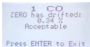
When the process has finished and the Zero calibration was accepted, press ENTER to Exit and remove the cylinder of zero gas. Refer to Section 7.3.3 *Zero - Requires Override* if the Zero calibration was not successful.
