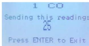
To stop the test, press ENTER to Exit. If you do not exit the test, the test will timeout after 5 minutes and return to normal operation. Repeat for each channel you want to test.
