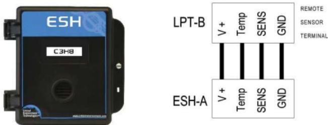
**The maximum length of wire between the ESH-A Remote Sensor and the transmitter should not exceed 61 m (200 ft).**
