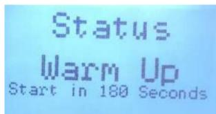
After the warm up period (3 minutes), the device may exhibit gas alarm conditions if the sensor has not completely stabilized during the warm up period. This is normal and the length of time the gas alarm exists is dependent upon the length of time since the unit was last powered up and the state of the environment it is installed in. Refer to Section 5 *Installation* for more information.
