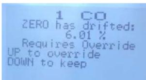
To override the value use the UP ARROW to select the desired value. To keep the original zero value, use the DOWN ARROW. Press ENTER to Exit.
