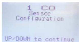
Press ENTER and use the ARROW keys to scroll through the menu and choose TEST. Press ENTER and use the ARROW key to increase or decrease the value and the ENTER key to move to the next digit.
