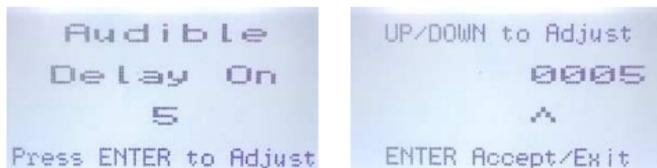
Press ENTER and use the ARROW keys to increase or decrease the number of seconds. Move to the next digit by pressing ENTER. When finished, press ENTER to save and Exit.
