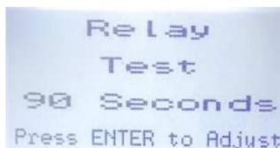
The test will start immediately and will continue for as long as the time was set. The remaining time of the test can be seen counting down on the display. You can exit the menu without affecting the time. **If you want to end the test before the time is up, you must re-enter the Test Mode and enter a value of "0000" for the test length of that function.**
