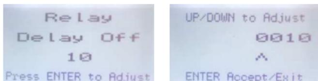
Press ENTER to access the screen and use the ARROW keys to increase or decrease the number. Press ENTER to move to the next digit and again to save and Exit the screen.
