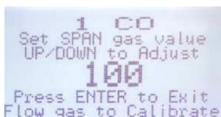
When the correct value is displayed, attach the regulator to the span gas cylinder and flow the span gas over the sensor. Once gas is detected, display will show a countdown from 180 seconds (3 minutes).
