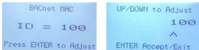
Press ENTER and use the ARROW keys to change the ID number. Move to the next digit by pressing ENTER. When finished, press ENTER to save and Exit.
