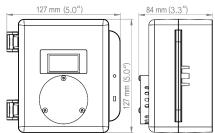
Note: Drawings above are shown with the optional splash guard. Without the splash quard, the thickness of the unit is 71 mm (2.8").
