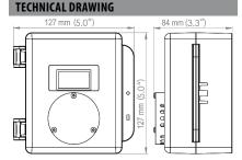
Note: Drawings above are shown with the optional splash quard. Without the splash guard, the thickness of the unit is 71 mm (2.8 inches).
