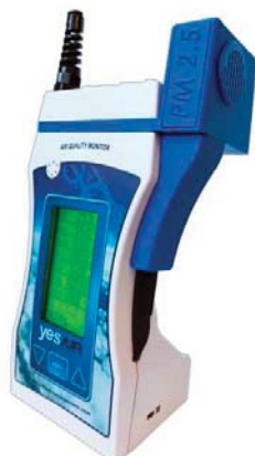
YESAIR shown with externally mounted particulate sensor
