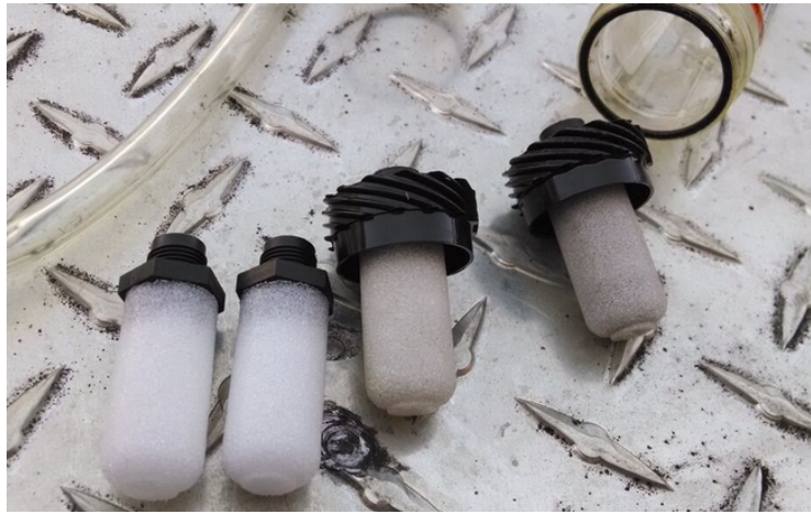
Fig. 12.B Clean and dirty filters
