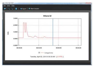
Downloaded data utilizing the Easylog software, is displayed in graphical form showing the peak(s) for the different gases in the sample taken. The sample above shows a typical natural gas sample indicating the date and time for each data point.
