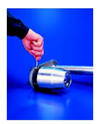
Place a piece of tracing paper in front of the receiver input lens and you will be able to see the rectangular shaped light beam projected onto the lens as well as the outline of the lens itself. If this light beam is not projecting onto the receiver lens at its center, adjust the alignment screws on the back of the light source until it is.
