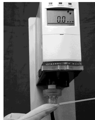
Block gas inlet
