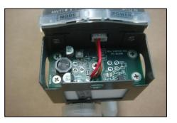
7. Re-fit the pyrolyzer case cover and push the cover lock knob upward. Switch the main unit power ON.
