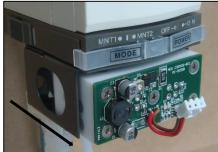
5. Exchange the pyrolyzer with a new one. The driver PCB is mounted with five screws.
