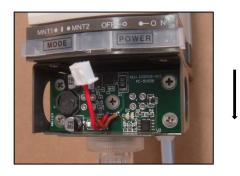
4. Hold the both sides of the pyrolyzer assembly, and remove it from the case.
