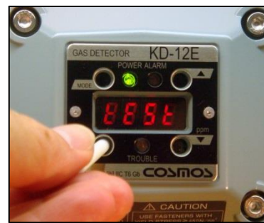
Figure 12-6: Test mode, TEST.
