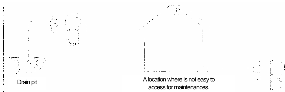
Fig.12 Example - location to install Suction type gas detector head
