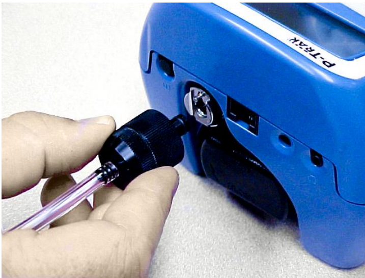
Figure 2-7: Insert Inlet Screen Assembly into Fitting
