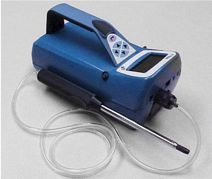
Figure 2-8: Slide Telescoping Probe onto Instrument Case
