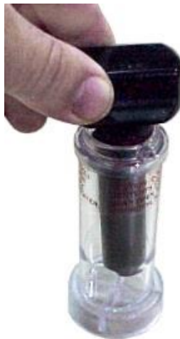
Figure 2-5: Insert Alcohol Cartridge into Fill Capsule
