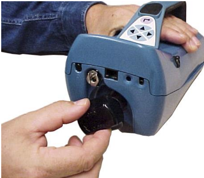
Figure 2-6: Insert Alcohol Cartridge into P-Trak Particle Counter
