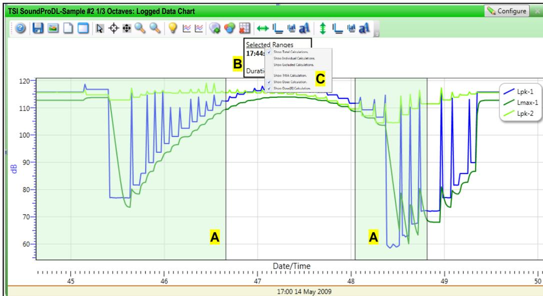
Figure 1-80: SoundPro meter and logged data chart with calculations
