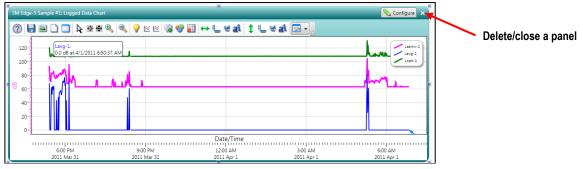
Figure 1-18: Deleting/closing data panels
