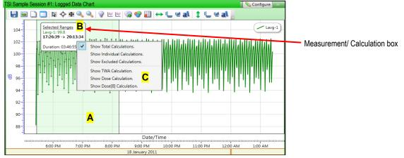
Figure 1-62: NoisePro dosimeter logged data chart and calculations
