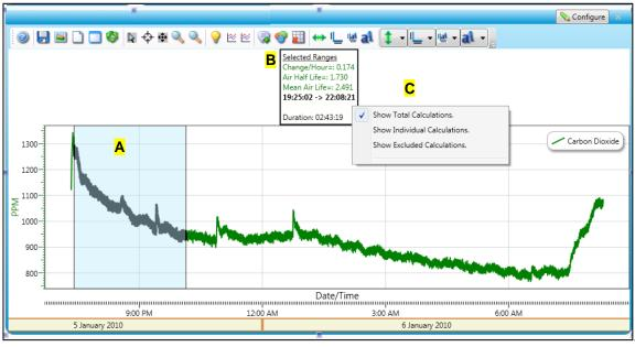
Figure 1-129: Logged data chart and selecting/recalculating
