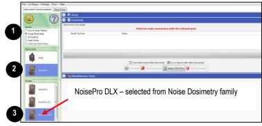
Figure 1-56: Instrument Communications/download layout
