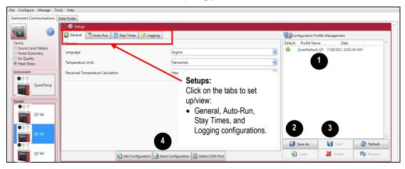
Figure 1-150: Saving and sending QUESTemp<sup>o</sup> 34/36 setups
