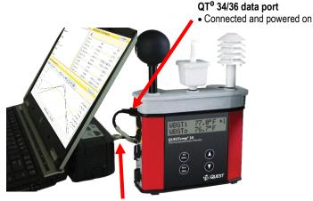
Connected to serial port
