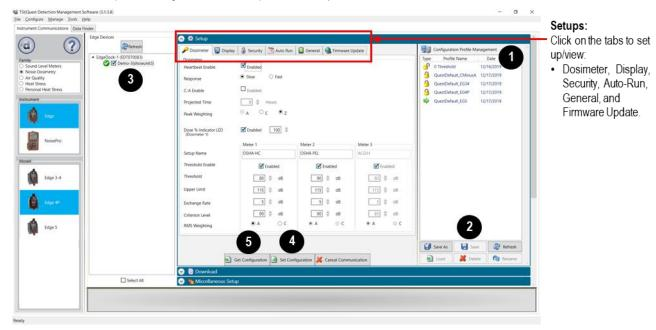
Figure 1-46: Saving and sending Edge setups
