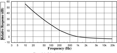
Figure A-1: C-A weighting response curve
