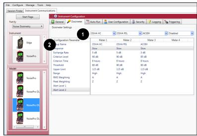
Figure 1-71: NoisePro dosimeter settings
