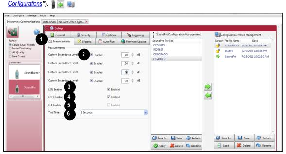
Figure 1-90: SoundPro Sound Level Meter measurement settings
