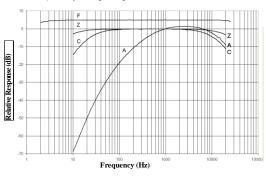
Figure A-6: All frequency weightings plotted together
