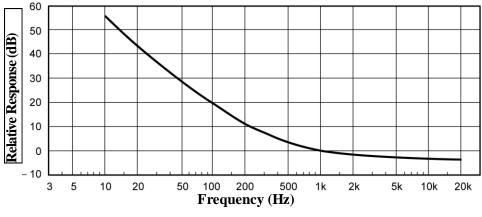
Figure A-2: C-A weighting response curve
