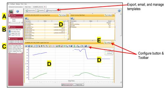
Figure 1-177: QUESTemp<sup>o</sup> II data in panel layout view
