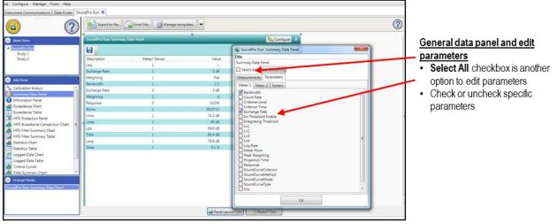
Figure 1-17: General data screen and selecting parameters via the configure icon.
