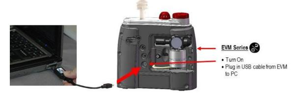
Figure 1-122: Communicating with the EVM and DMS
