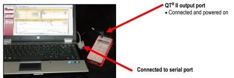
Figure 1-173: Communicating with the QUESTemp<sup>o</sup> II and DMS
