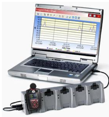
Figure 5-1 Communicating Between your PC and the Edge
