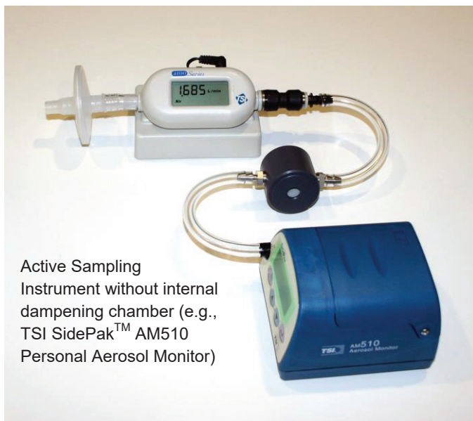
Figure 2-3 Typical Dampening Module Set Up
