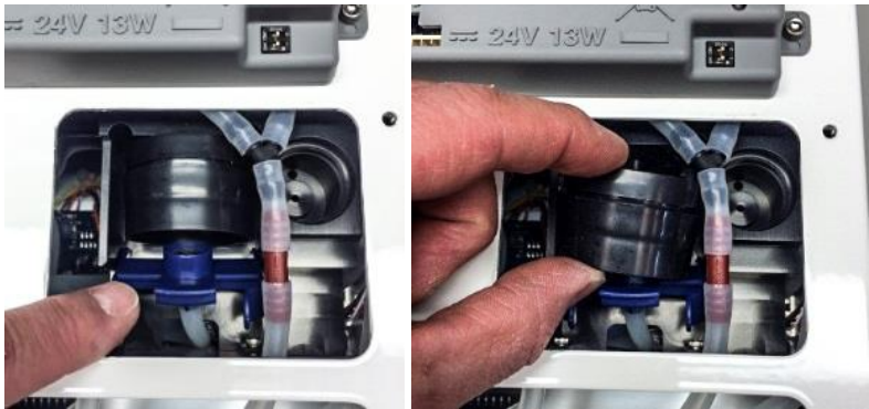
Figure 33: Release and remove cassette holder
