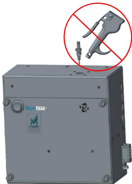
Figure 18: DO NOT Blow into Instrument
