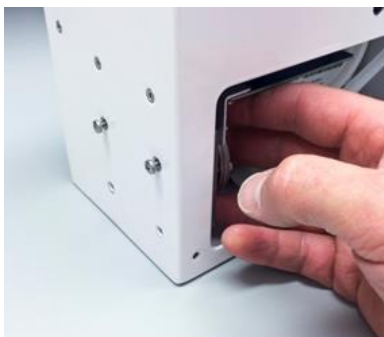
Figure 31: Secure new pump
