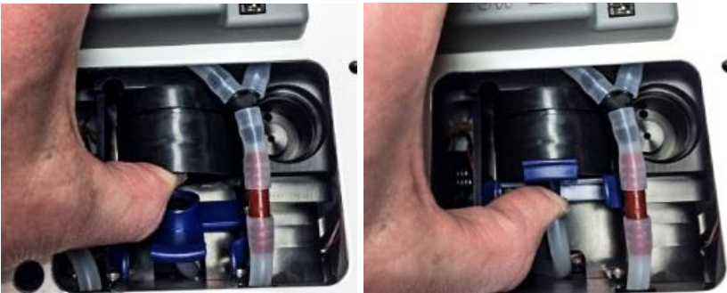
Figure 35: Snap cassette securely into inlet port
