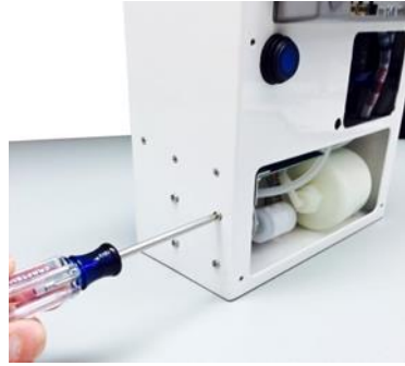
Figure 27: Remove screws from left side panel
